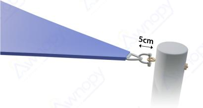
Leave a 5 cm gap between the two anchor points where the D-shackles will be attached. This allows for proper installation.
